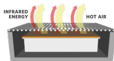
Other infrared grills use TEC's old ceramic infrared burners. Grates are heated unevenly, and although they cook hot and fast, they cannot cook at the lower temperatures needed for delicate foods, smoking, or barbecuing.
